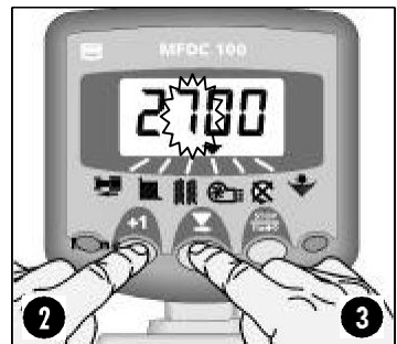
Figure 17: Low speed alarm threshold
