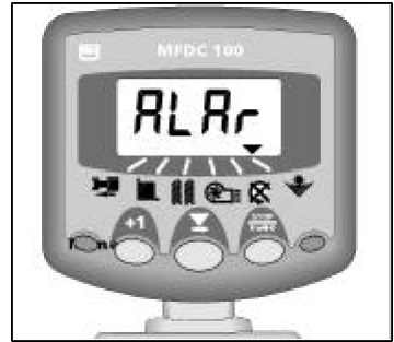
Figure 20: Hopper Low Alarm
